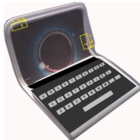
Fig. 1. Typical placement and embedding of the flexible antenna onto a flexible and potentially rollable display screen of a commercially available laptop. The antenna locations are shown with dashed and dotted lines. The original screen capture is from [6].
